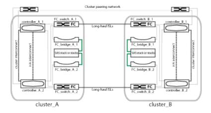
The following illustration shows a more detailed view of the connectivity in a single MetroCluster cluster (both clusters have the same configuration):
