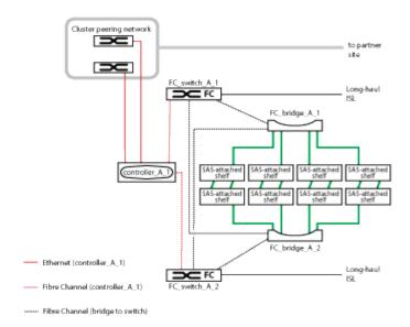
A two-node configuration includes the following connections:
