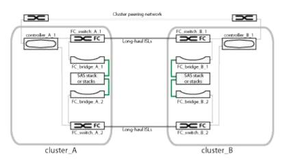
A two-node configuration consists of two clusters, one at each geographically separated site. cluster\_A is located at the first MetroCluster site. cluster\_B is located at the second MetroCluster site. Each site has one SAS storage stack. Additional storage stacks are supported, but only one is shown at each site.
