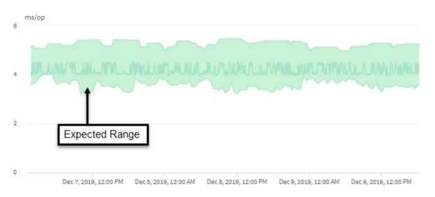
In this example, the latency for a volume has a latency forecast, in gray, of 3.5 milliseconds per operation
