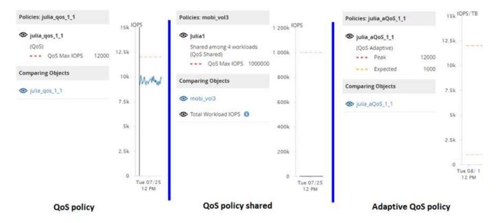
When a normal QoS policy that has been defined in IOPS appears in the IOPS/TB chart for a workload, ONTAP converts the IOPS value to an IOPS/TB value and Unified Manager displays that policy in the IOPS/TB chart along with the text "QoS, defined in IOPS".
