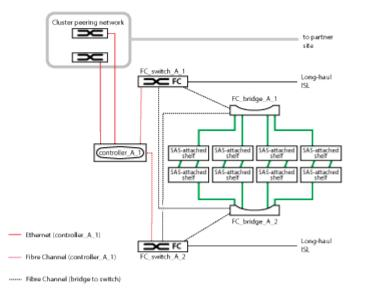
A two-node configuration includes the following connections:
