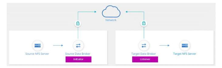
One data broker functions as the *initiator*. When it's time to sync data, it sends a connection request to the other data broker, which is the *listener*. That data broker listens for requests on port 443. You can use a different port, if needed, but be sure to check that the port is not in use by another service.
