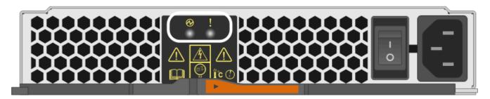
If the Power LED is **solid green**, the power supply is functioning correctly. If it is **Off**, the power supply failed, the AC switch is turned off, the AC power cord is not properly installed, or the AC power cord input voltage is not within margin (there is a problem at the source end of the AC power cord).
