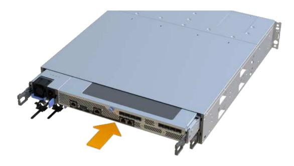
Install the SFPs into the new HIC and reconnect all the cables.
