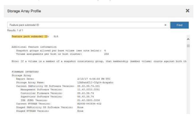
Using the feature pack submodel ID, locate the corresponding Controller submodel ID for the starting configuration and find the Feature Activation Code for the desired ending configuration within the following
