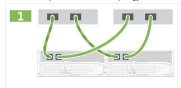
1. Connect each host adapter directly to the host ports on the controllers.
