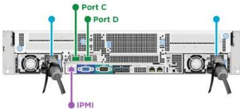
Here are the network ports and locations on the H615C compute node:
