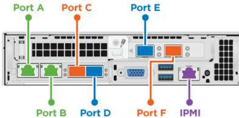
Here are the network ports and locations on the H610C compute node:
