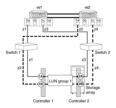
In this configuration with a single 4-port LUN group, array LUNs are mapped to four ports on the storage array. The array LUN group is presented to both nodes in the HA pair on different array target ports. However, each node can see an array LUN, end-to-end, through only two paths. Zoning is configured so that each FC initiator port on a node can access only a single target array port.
