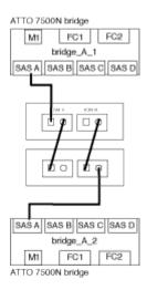
2. For additional shelf stacks, repeat the previous steps using the next available SAS port on the FibreBridge bridges, using port B for a second stack, port C for a third stack, and port D for a fourth stack.
