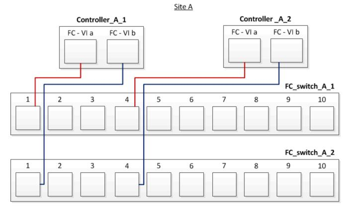
2. Perform the controller-to-switch cabling at both of the MetroCluster sites.
