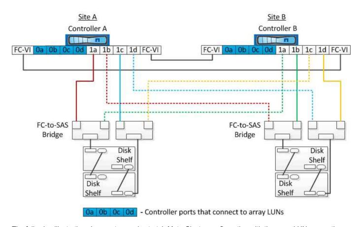
The following illustration shows a two-node stretch MetroCluster configuration with the array LUN connections:
