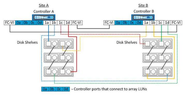
The following illustration shows a two-node stretch MetroCluster configuration in which the native disks are connected to the ONTAP systems using FC-to-SAS bridges:
