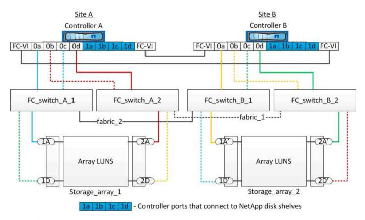
If required, you can also use the same FC switches to connect both native disks and array LUNs to the controllers in the MetroCluster configuration.
