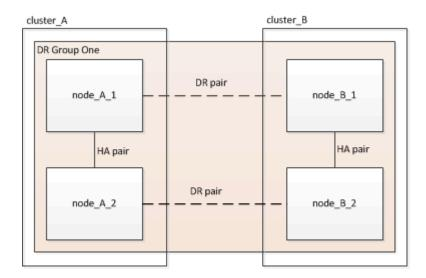
At the conclusion of this procedure, the MetroCluster FC configuration consists of two HA pairs at each site:
