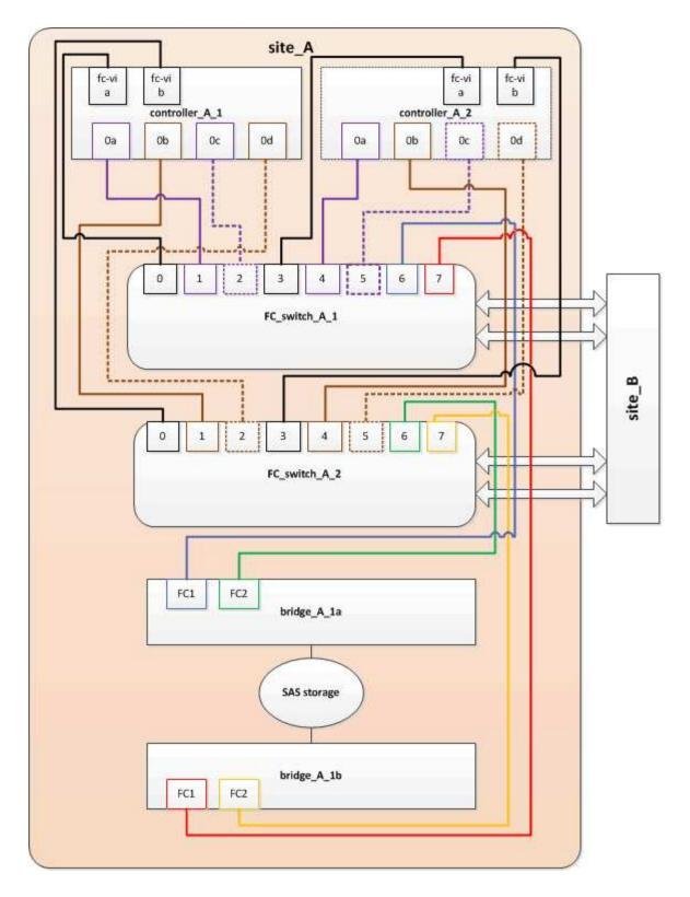
Updating zoning when adding FibreBridge 7600N or 7500N bridges to a configuration (ONTAP 9.1 and later)
