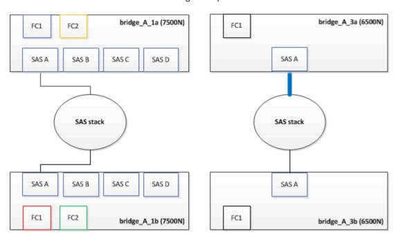
2. Using a cable with a mini-SAS connector, connect the same SAS port on the storage shelf to the SAS B port of the top FibreBridge 7600N or 7500N bridge.
