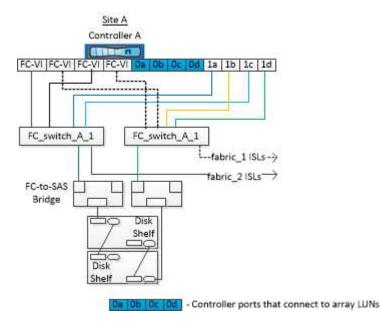
In the following illustration showing the connectivity between ONTAP systems and array LUNs, the HBA ports 0a through 0d are used for connectivity with array LUNs because ports 1a through 1d are used for connectivity with disks:
