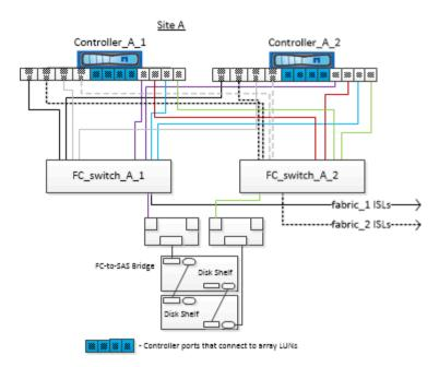
In the following illustration that shows the connectivity between ONTAP systems and array LUNs, the HBA ports 0a through 0d are used for connectivity with array LUNs because ports 1a through 1d are used for connectivity with disks:
