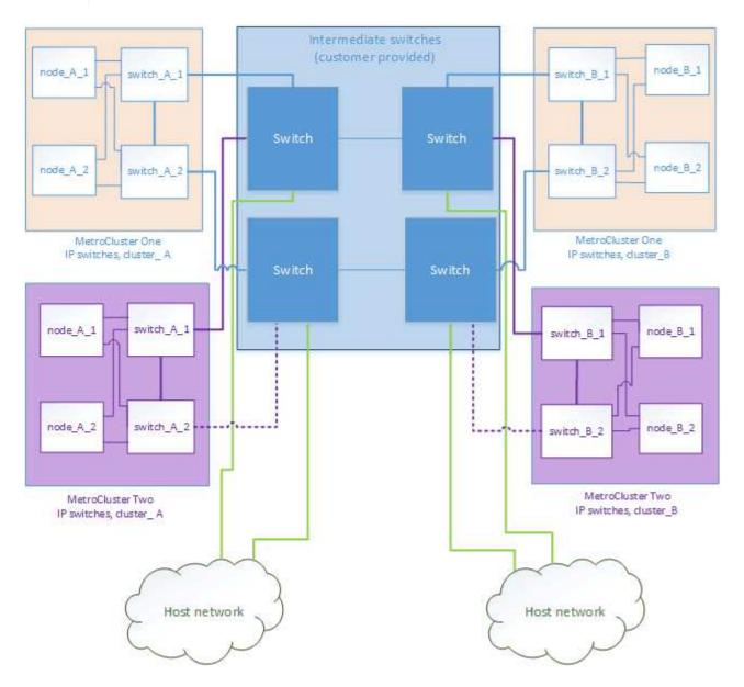
Combination of a MetroCluster configuration using NetApp validated switches and a configuration using MetroCluster-compliant switches
