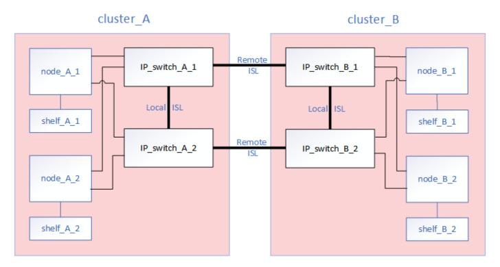
Each node in the MetroCluster IP configuration has specialized LIFs for connection to the back-end IP network:
