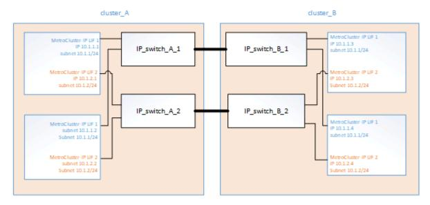
The MetroCluster IP configuration requires two IP addresses on each node that are reserved for the back-end MetroCluster IP fabric. The reserved IP addresses are assigned to MetroCluster IP logical interfaces (LIFs) during initial configuration, and have the following requirements:
