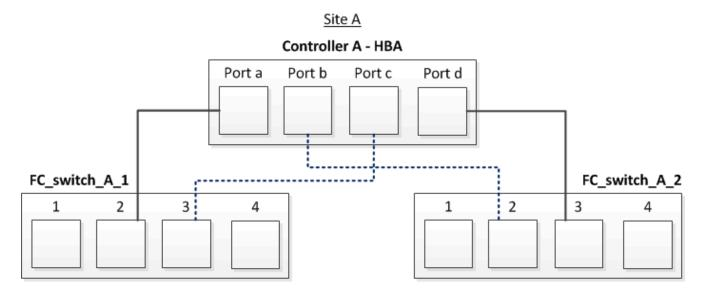
The following table lists the connections between the HBA ports and the FC switch ports in the illustration:
