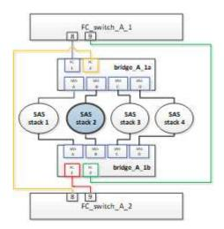
SAS port B connects the bridges to the target shelf. By disabling only SAS port B on both shelves, the other SAS stacks can continue to serve data during the replacement procedure.
