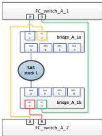
Switch ports 8 and 9 on each switch connect the bridges to the network.
