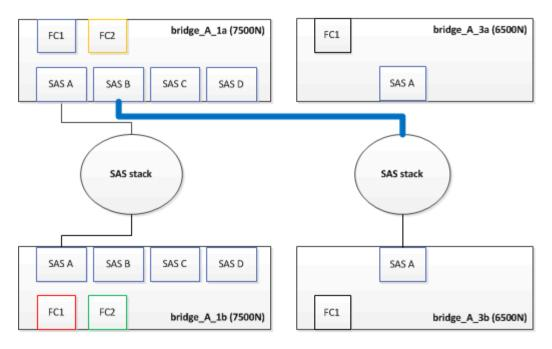
3. Remove the cable that connects the SAS A port of the bottom FibreBridge 6500N bridge to the top SAS shelf, being sure to note the SAS port on the storage shelf to which it connects.
