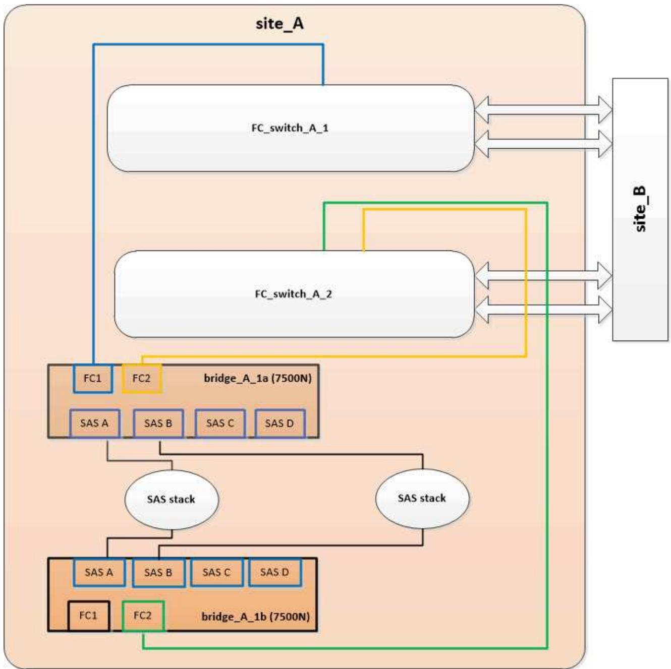
2. Cable the FC1 port of the bottom bridge to the correct port on FC\_switch\_A\_1.
