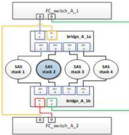
SAS port B connects the bridges to the target shelf. By disabling only SAS port B on both shelves, the other SAS stacks can continue to serve data during the replacement procedure.
