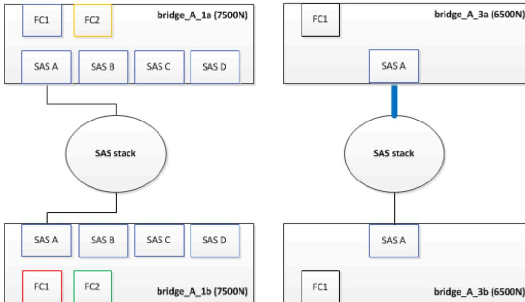
2. Using a cable with a mini-SAS connector, connect the same SAS port on the storage shelf to the SAS B port of the top FibreBridge 7600N or 7500N bridge.
