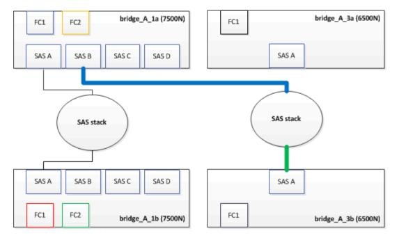
4. Using a cable with a mini-SAS connector, connect the same SAS port on the storage shelf to the SAS B port of the bottom FibreBridge 7600N or 7500N bridge.
