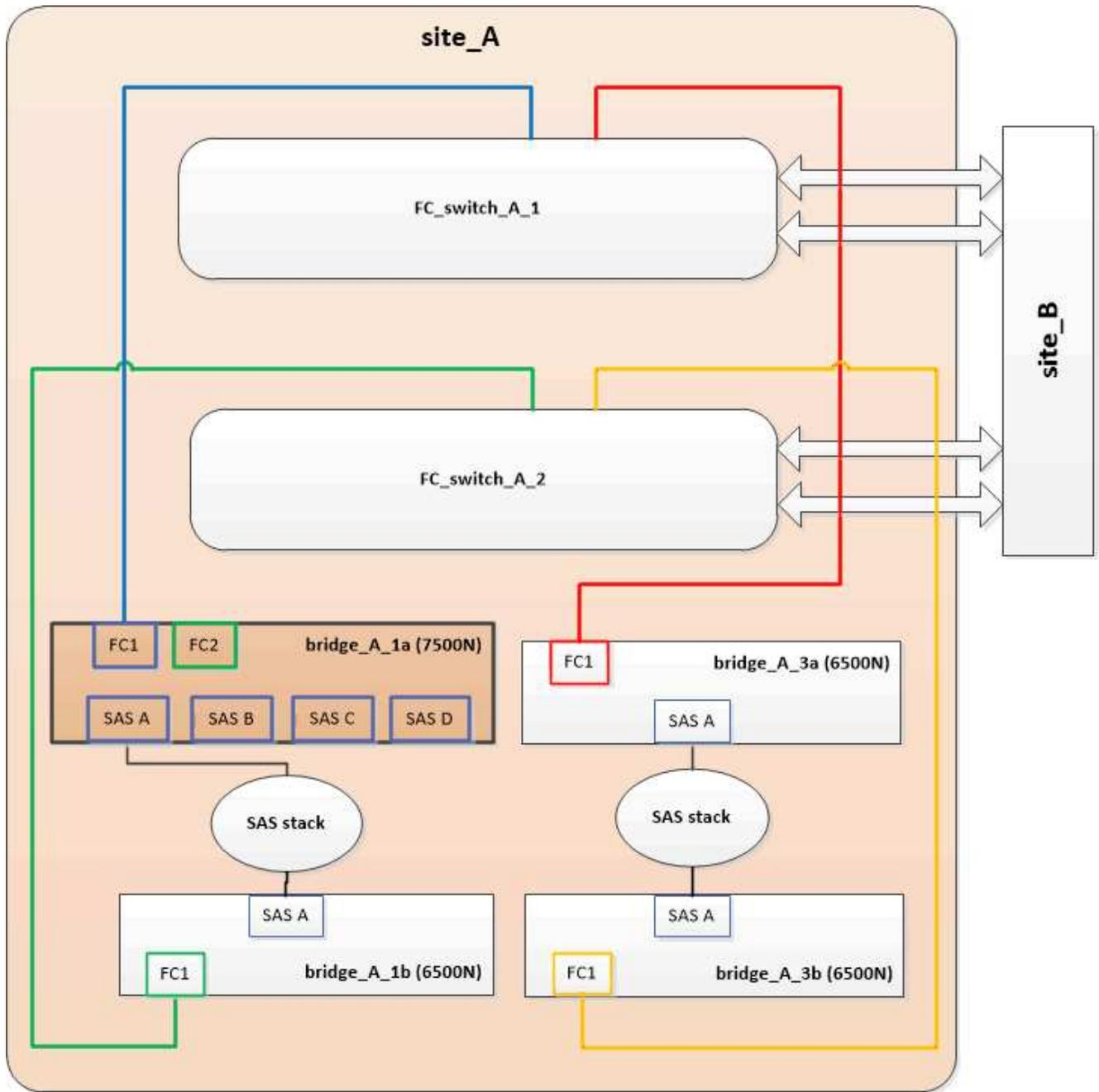
2. Confirm connectivity to the bridge-connected disks and that the new FibreBridge 7500N is visible in the configuration:
