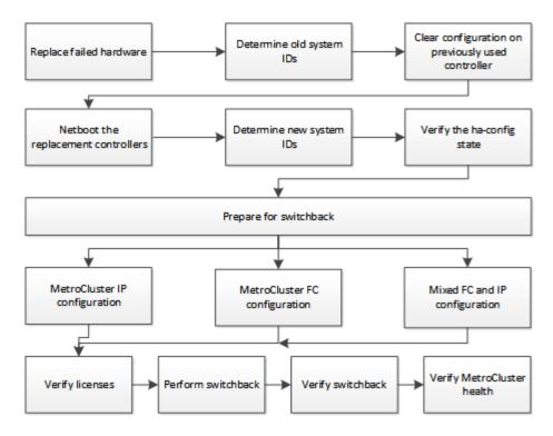
This procedure can be used when performing recovery on a system that was in mid-transition when the failure occurred. In that case, you must perform the appropriate steps when preparing for switchback, as indicated in the procedure.
