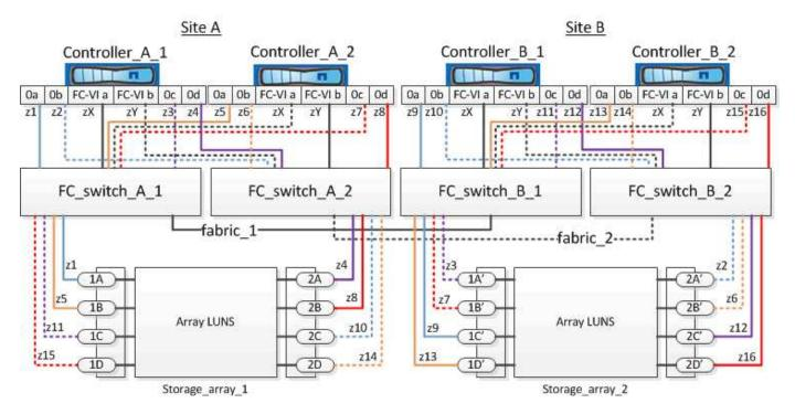
In the illustration, array LUNs are allocated on each storage array for the MetroCluster configuration. LUNs of equal size are provisioned on the storage arrays at both sites, which is a SyncMirror requirement. Each ONTAP system has two paths to array LUNs. The ports on the storage array are redundant.
