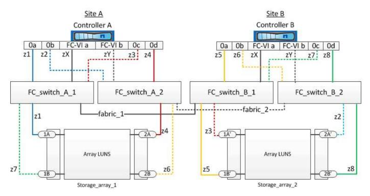
The example shows single-initiator to single-target zoning for the MetroCluster configurations. The lines in the example represent zones rather than connections; each line is labeled with its zone number.
