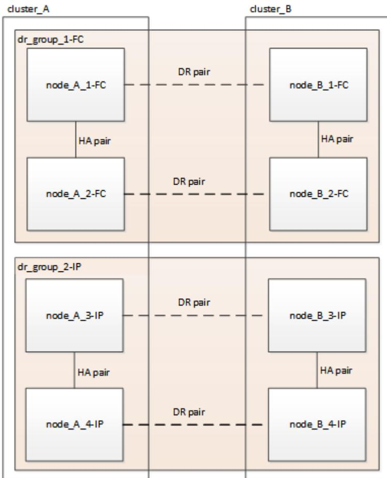
Data is transferred from the old DR group to the new DR group, and then the old nodes and their storage are removed from the configuration and decommissioned. The process ends with a four-node MetroCluster IP configuration.
