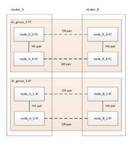
Add the remaining MetroCluster IP nodes to the existing MetroCluster configuration. Repeat the process to transfer data from the DR\_group\_2-FC nodes to the DR\_group\_2-IP nodes.
