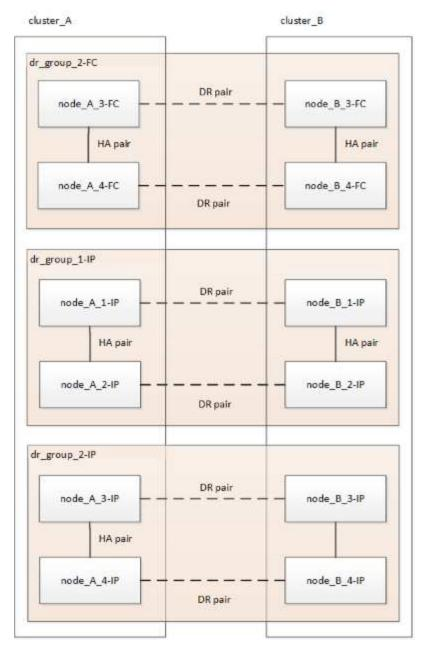
After removing DR\_group\_2-FC, the process ends with an eight-node MetroCluster IP configuration.
