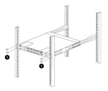
(1) With one person holding the front of the chassis level, the other person should fully tighten the four rear screws to the cabinet posts.
