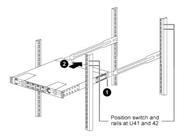
(1) As the chassis is pushed toward the rear posts, align the two rear rack-mount guides with the slider rails.
