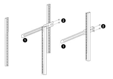
(1) As you gently slide the slider rail, align it to the screw holes in the rack.(2) Tighten the screws of the slider rails to the cabinet posts.
