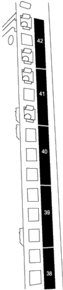
The two 9336C-FX2 switches will always be mounted in the top 2U of the cabinet RU41 and 42.
