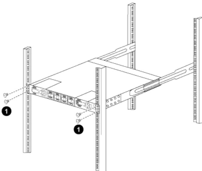
(1) With one person holding the front of the chassis level, the other person should fully tighten the four rear screws to the cabinet posts.
