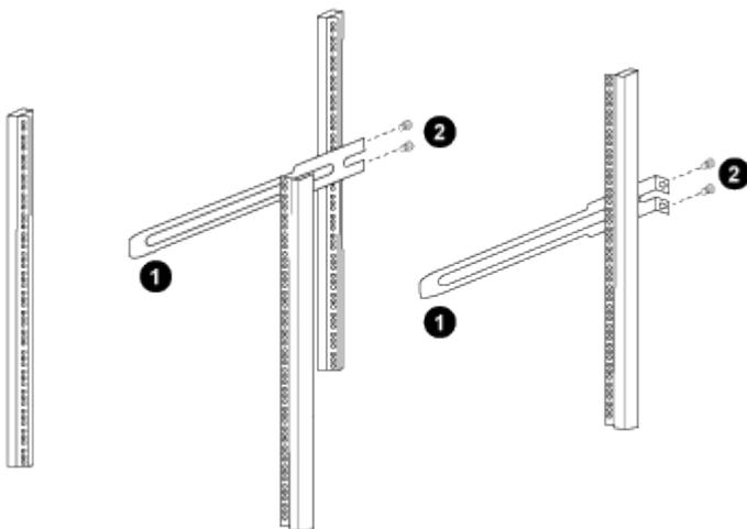
*(1) As you gently slide the slider rail, align it to the screw holes in the rack.*
