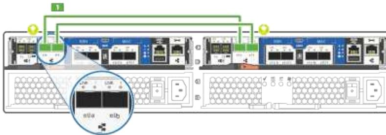
2. Cable the controllers to either a UTA2 data network or an Ethernet network:
