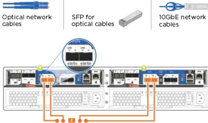
You can connect one port pair as CNA and one port pair as FC, or you can connect both port pairs as CNA or both port pairs as FC.
