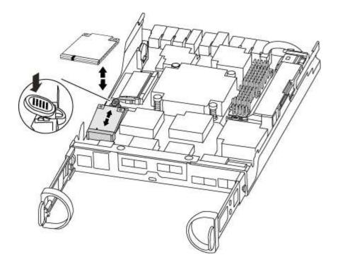
3. Press the blue button on the boot media housing to release the boot media from its housing, and then gently pull it straight out of the boot media socket.
