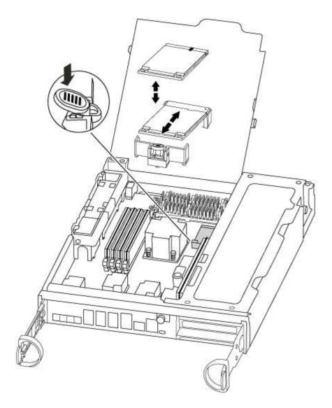
3. Press the blue button on the boot media housing to release the boot media from its housing, and then gently pull it straight out of the boot media socket.
