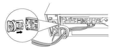
4. Loosen the thumbscrew on the cam handle on the controller module.
