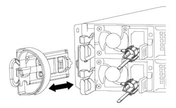
Leave the cables in the cable management device so that when you reinstall the cable management device, the cables are organized.
