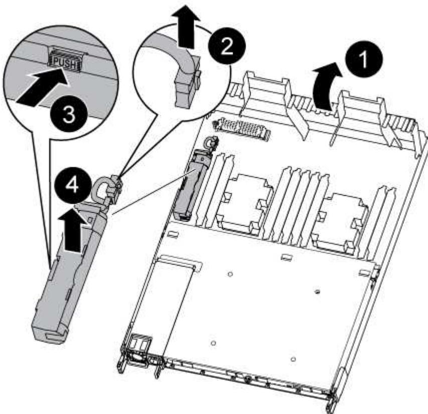
1. Open the air duct and locate the NVDIMM battery.
