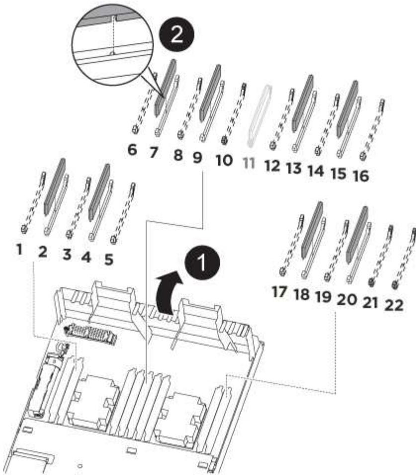
1. Locate the DIMMs on your controller module.
