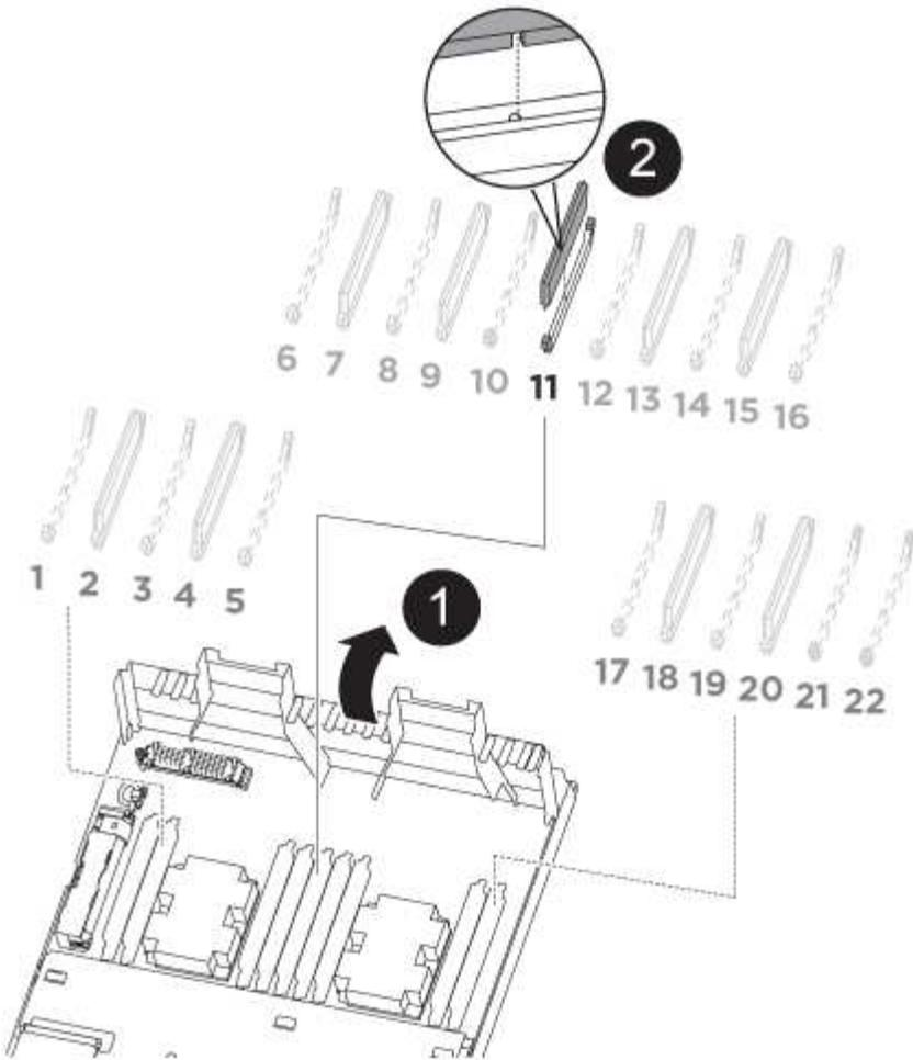
1. Open the air duct and then locate the NVDIMM in slot 11 on your controller module.
