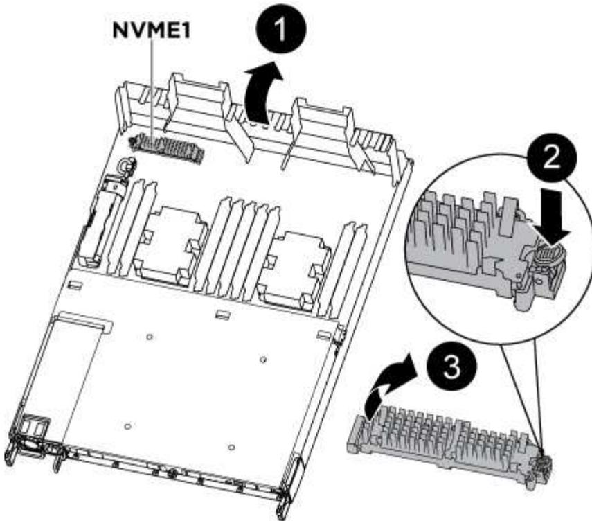
1. Open the air duct and locate the boot media using the following illustration or the FRU map on the controller module:
