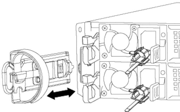
Leave the cables in the cable management device so that when you reinstall the cable management device, the cables are organized.
