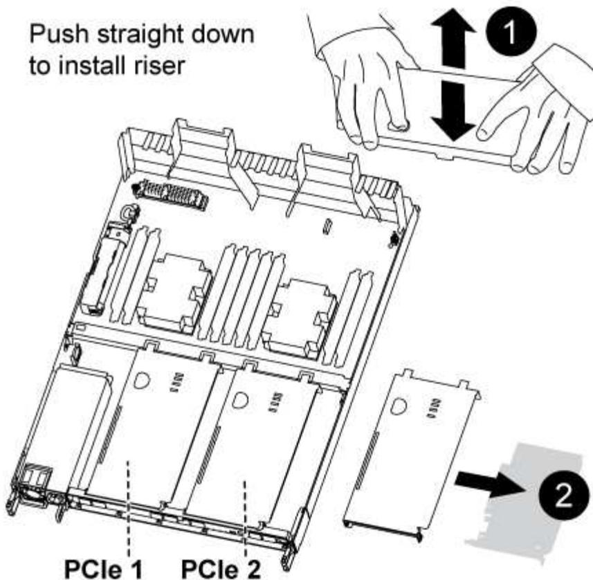
1. Remove the cover over the PCIe risers by unscrewing the blue thumbscrew on the cover, slide the cover toward you, rotate the cover upward, lift it off the controller module, and then set it aside.
