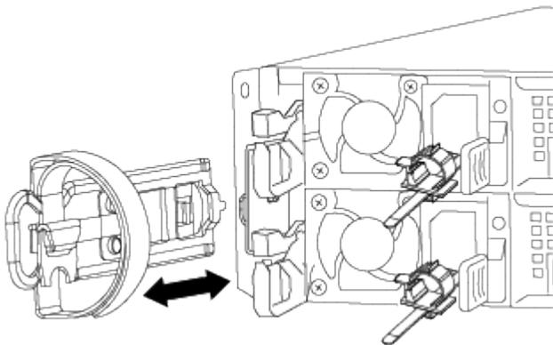
The following image shows removing the impaired controller module from the chassis:
