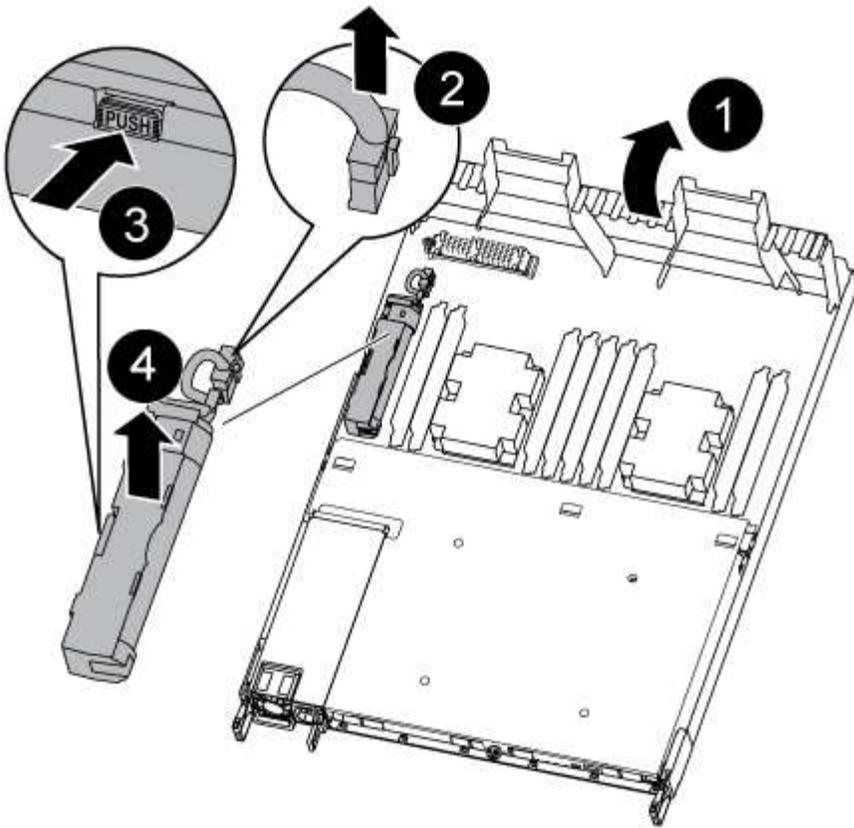
1. Locate the NVDIMM battery in the controller module.
