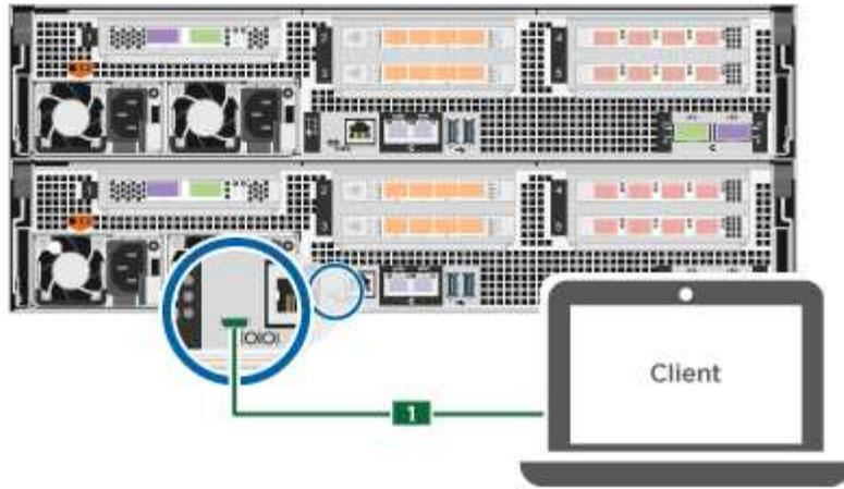
c. Connect the laptop or console to the switch on the management subnet.
