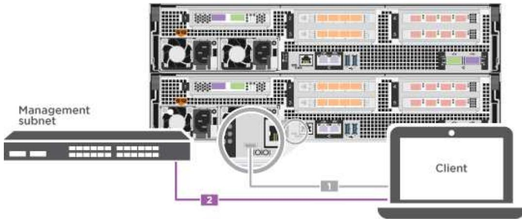
d. Assign a TCP/IP address to the laptop or console, using one that is on the management subnet.
