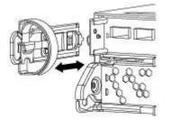
4. Squeeze the latch on the cam handle until it releases, open the cam handle fully to release the controller module from the midplane, and then, using two hands, pull the controller module out of the chassis.
