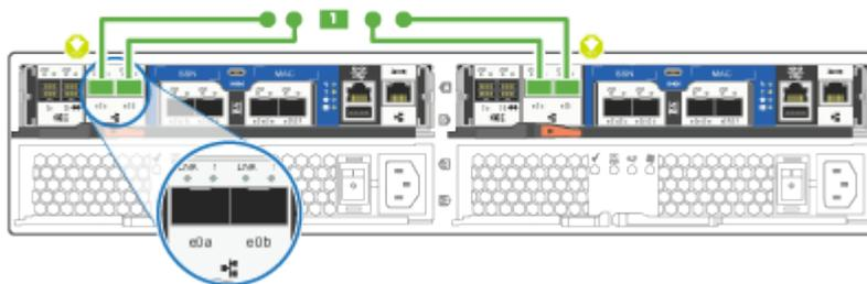
2. Cable the controllers to either a UTA2 data network or an Ethernet network.
