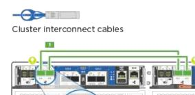
2. Cable the controllers to either a UTA2 data network or an Ethernet network.
