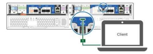
c. Connect the laptop or console to the switch on the management subnet.
