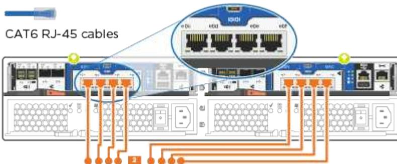
3. Cable the e0M ports to the management network switches with the RJ45 cables.
