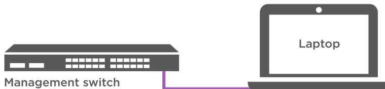
c. Assign a TCP/IP address to the laptop or console, using one that is on the management switch.
