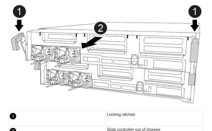
6. Slide the controller module out of the chassis.
