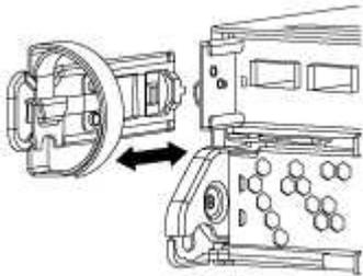
3. Squeeze the latch on the cam handle until it releases, open the cam handle fully to release the controller module from the midplane, and then, using two hands, pull the controller module out of the chassis.
