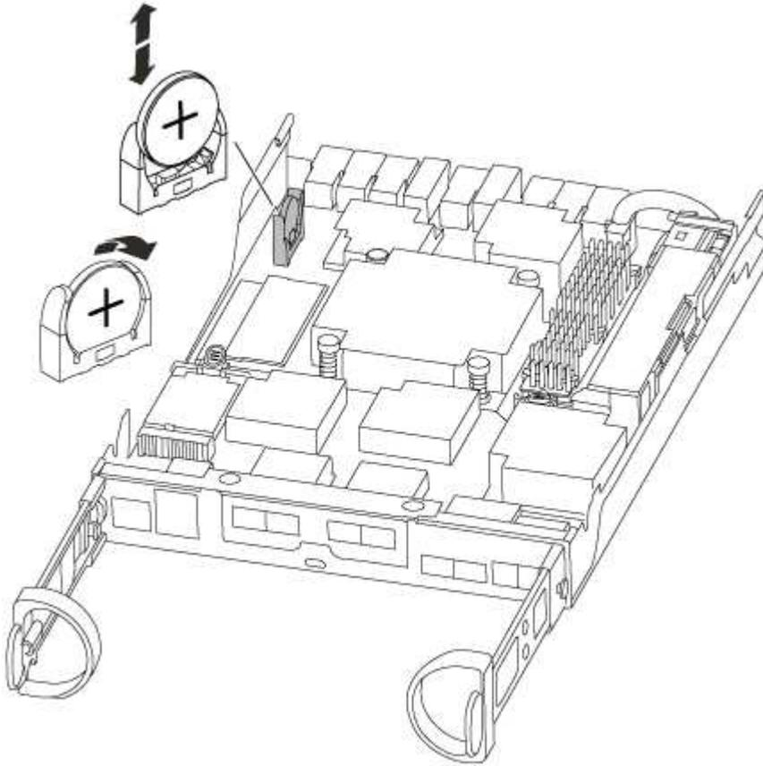
3. Gently push the battery away from the holder, rotate it away from the holder, and then lift it out of the holder.
