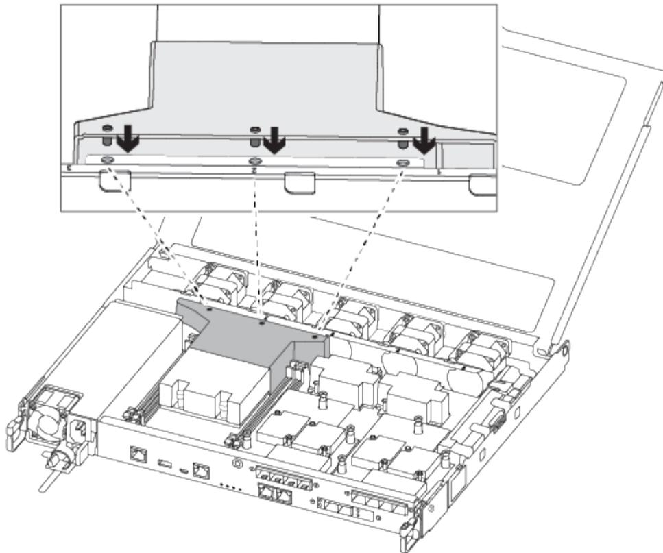
2. Close the controller module cover and tighten the thumbscrew.
