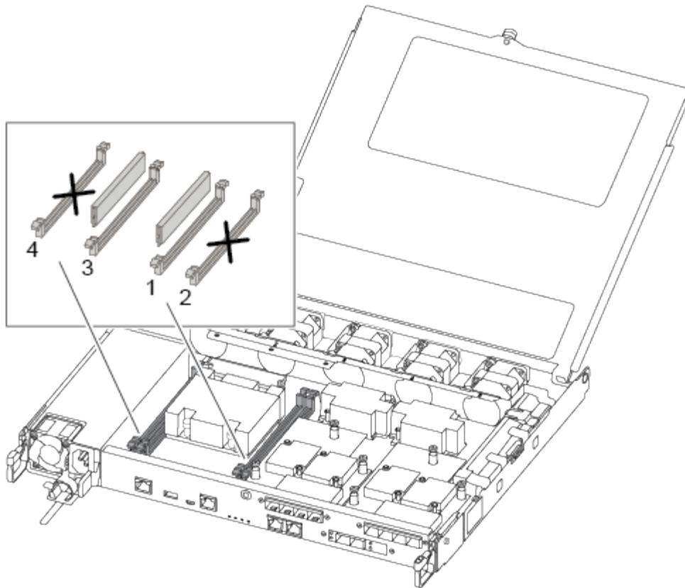
2. Note the orientation of the DIMM in the socket so that you can insert the replacement DIMM in the proper orientation.
