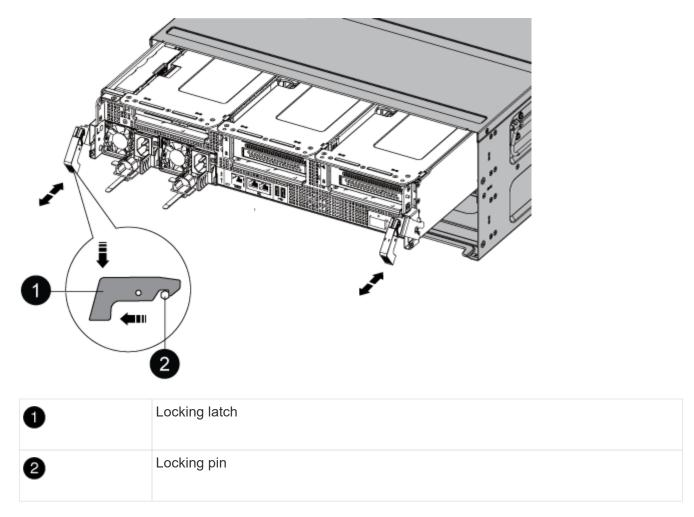
7. Slide the controller module out of the chassis.
