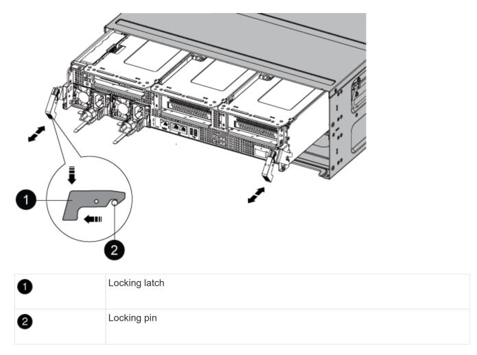
8. Slide the controller module out of the chassis and place it on a stable, flat surface.
