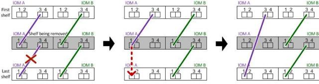
Verify that you bypassed the disk shelves you are removing and reestablished the path A (IOM A) stack connections correctly: storage disk show -port
