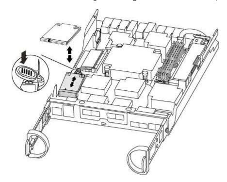
3. Press the blue button on the boot media housing to release the boot media from its housing, and then
