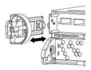
4. Squeeze the latch on the cam handle until it releases, open the cam handle fully to release the controller module from the midplane, and then, using two hands, pull the controller module out of the chassis.
