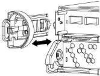
4. If you left the SFP modules in the system after removing the cables, move them to the new controller module.
