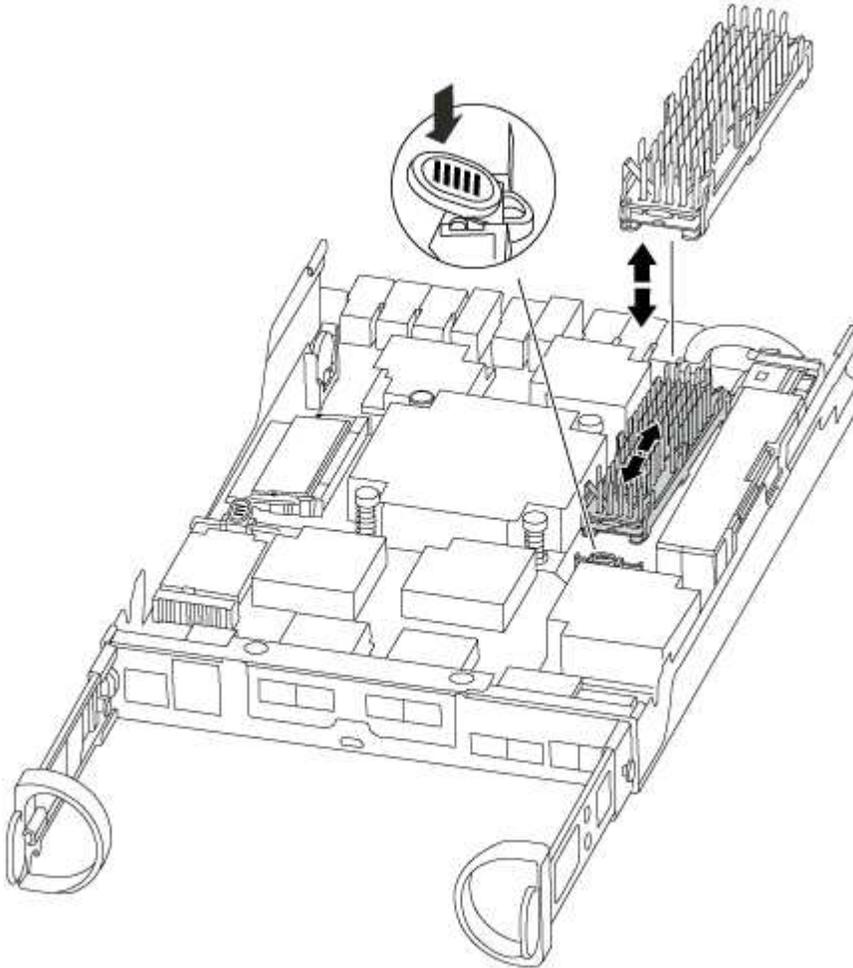
1. Gently pull the caching module straight out of the housing.
