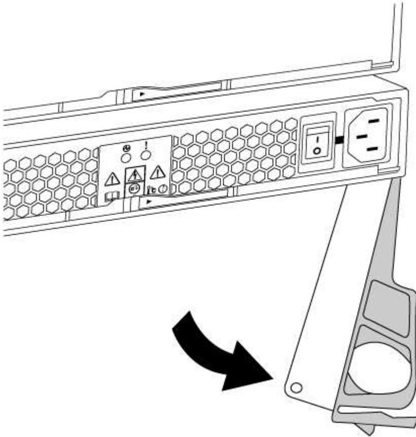
5. Use the cam handle to slide the power supply out of the system.
