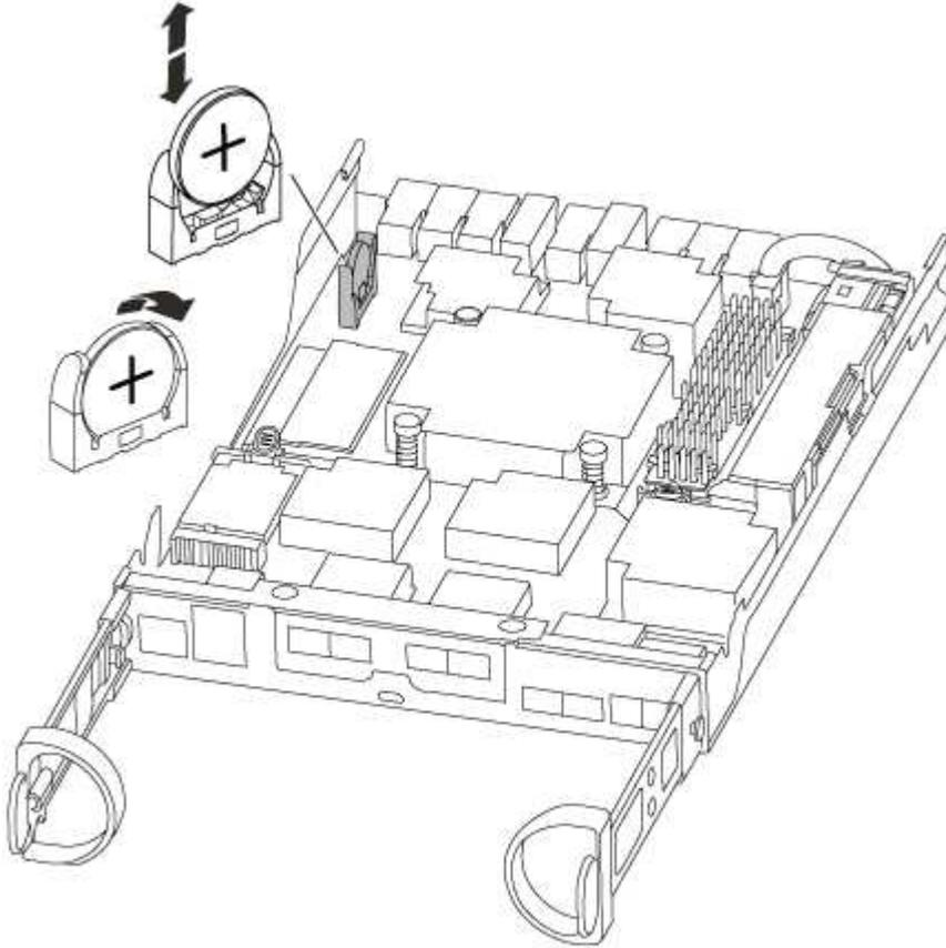
2. Gently push the battery away from the holder, rotate it away from the holder, and then lift it out of the holder.
