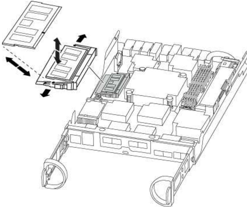
8. Remove the replacement DIMM from the antistatic shipping bag, hold the DIMM by the corners, and align it to the slot.
