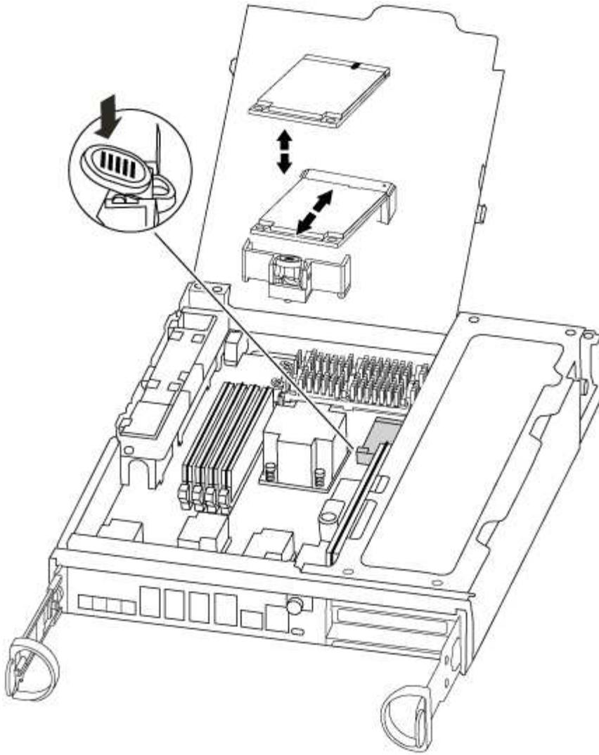
3. Press the blue button on the boot media housing to release the boot media from its housing, and then gently pull it straight out of the boot media socket.
