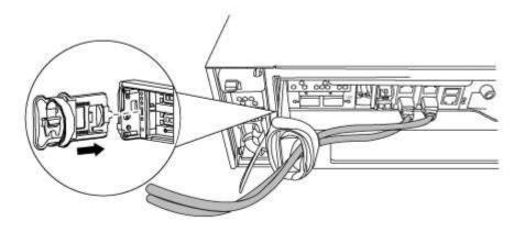
4. Loosen the thumbscrew on the cam handle on the controller module.
