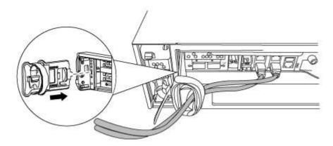
3. Loosen the thumbscrew on the cam handle on the controller module.
