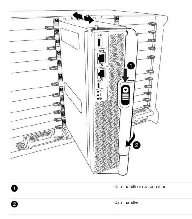
4. Rotate the cam handle so that it completely disengages the controller module from the chassis, and then slide the controller module out of the chassis.
