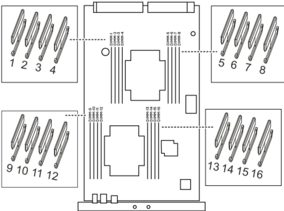
1. Eject the DIMM from its slot by slowly pushing apart the two DIMM ejector tabs on either side of the DIMM, and then slide the DIMM out of the slot.
