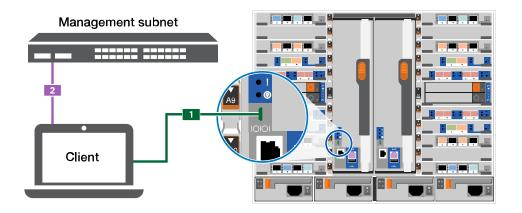
c. Assign a TCP/IP address to the laptop or console, using one that is on the management subnet.
